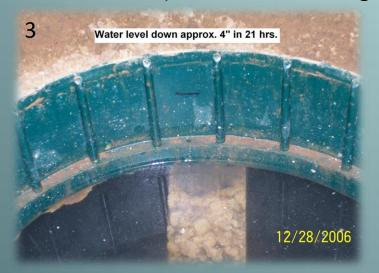
No water was used in the home during the leak test, which confirmed the tank was leaking.
